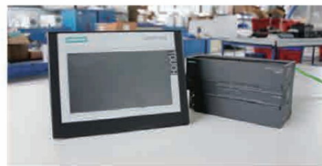
SIEMENS PLC & Touch Screen
