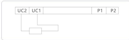
M1 series moulded case circuit breaker undervoltage release wiring diagram
