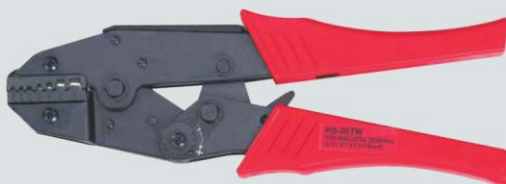
HS-26TW Cable range:0.5-6mm 2
