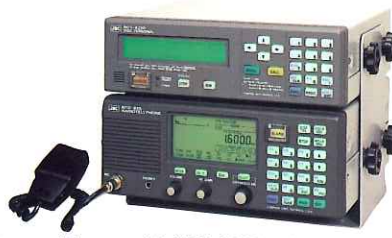
(Upper unit) NCT-620D DSC terminal (Lower unit) NTD-825 transmitter/receiver
