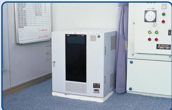
Photo: VDR on board "Pacific Venus" by courtesy of Japan Cruise Line, Inc.
