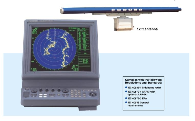
The FR-2135S and FR-2165DS are designed for a wide range of users such as coasters, fishing boats, yachts, cargo ships and passenger ships requiring a second radar or 10 cm radar features. The S-band radar assures target detection in adverse weather where X-band radars are heavily affected by sea or rain clutter. It is recommended that the vessel install both X-band and S-band radars.
