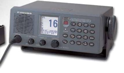
The FURUNO FM-8800S/8800D are high quality, all-in-one marine VHF radiotelephones designed to comply with the GMDSS carriage requirements for safety and general communications. All the necessary functions such as a 25 W VHF radiotelephone, a Class A DSC modem and a CH 70 Watch Receiver are incorporated into the compact transceiver unit.
