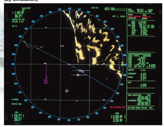
The AIS enhances detection of other ships and AtoN (aids to navigation) on radar screen.
