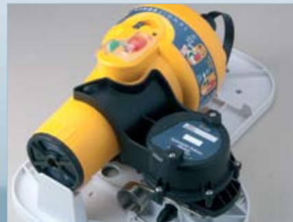
EPIRB Mounted with hydrostatic release
