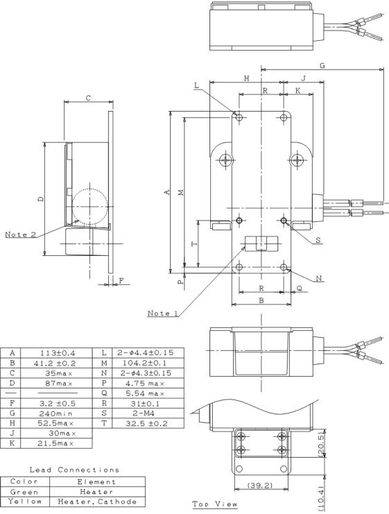
Note 1:The position of the waveguide and fixing holes will be such that the valve operates into coupler type UG-40 B/U. Note 2:Anode temperature mesured at this point.
