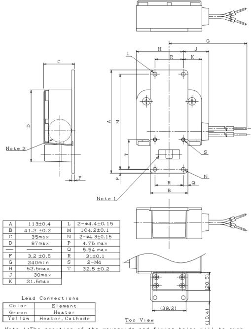
Note 1:The position of the waveguide and fixing holes will be such that the valve operates into coupler type UG-40 B/U. Note 2:Anode temperature mesured at this point.
