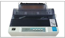
PP550/NKG950 printer is required for the Class 1 configuration. The PP550/NKG950 is a serial dot matrix impact printer; all incoming and outgoing telex messages are automatically printed.
