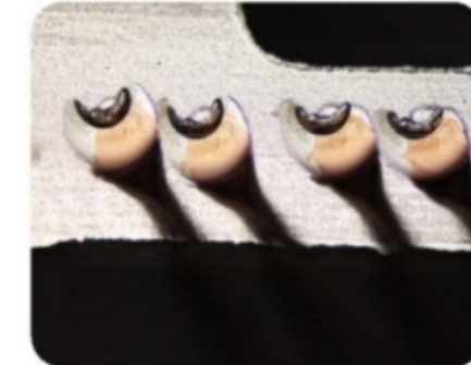
一普银线稳定的第二焊点 The internal organization of the second solder spot is uniform
