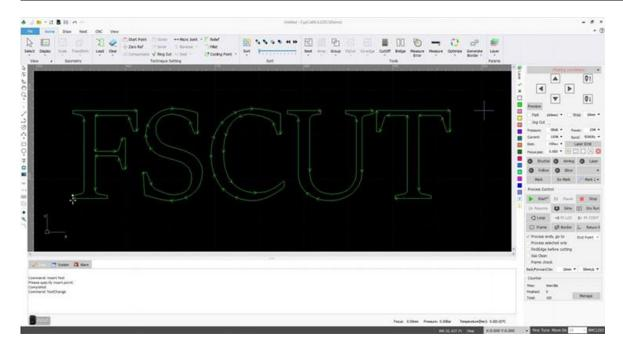
The FSCUT system is a very popular operating system for professional laser cutting machines. It is easy to install and debug, has excellent performance and provides a complete solution. The system has functions such as automatic edge finding, common edge cutting, perforation and slag removal, compensation function, thin plate flying cutting, fault self-detection, automatic conversion of CAD drawings, and automatic memory.
