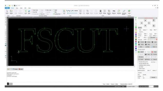
The FSCUT system is a very popular professional laser cutting machine operating system. It is easy to install and debug, with excellent performance and provides a complete solution. The system has functions such as automatic edge finding, common edge cutting, perforation slag removal, compensation, thin plate flying cutting, fault self detection, CAD drawing automatic conversion, and automatic memory.
