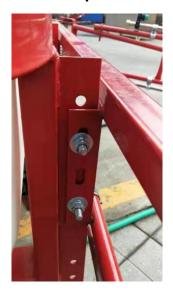
3. 连接喷药管和喷头、将喷头固定在不锈钢管合适位置上,用喷药管件连接喷头并紧好以防滴漏。Connect the spray nozzle and the spray tube, fix the spray nozzle in the appropriate position of the
