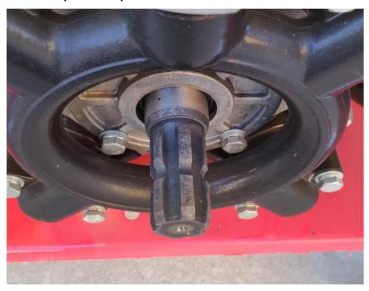
11. 使用三点悬挂挂接在拖拉机后方。传动轴万向节两端必须要用固定插销及锁紧螺栓固定锁紧。Use three-point suspension to attach to the rear of the tractor. Both ends of the universal joint of the PTO shaft must be fixed and locked with fixed bolt.
