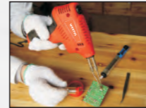
Area B: 200°C-350°C Normal soldering
