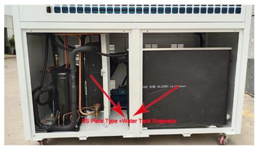
SS Plate Type+ Water Tank Evaporator
