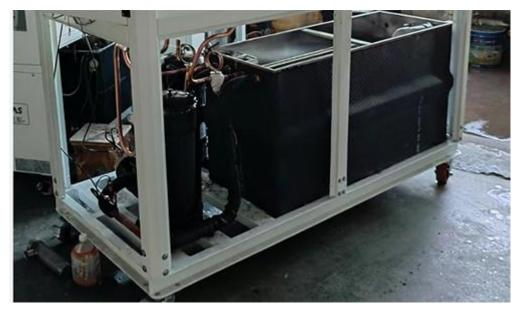
Coil in SS Water Tank Evaporator
