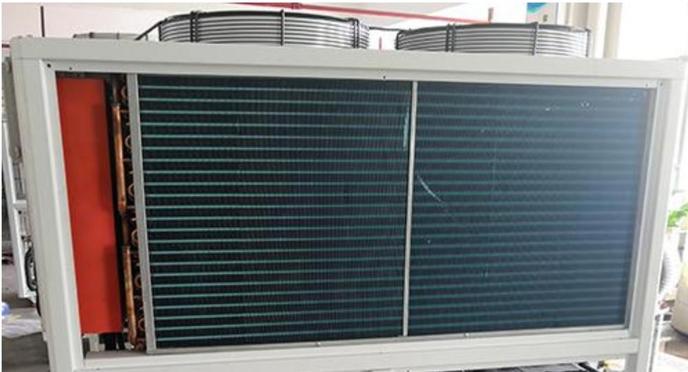
*Aluminum fin+fan Condenser for air -cooled plasma cutting chiller*
