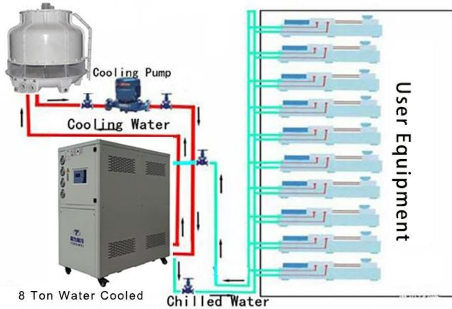
**8 Ton Water Cooled Chiller with Water Tank And Water Pump Inside**
