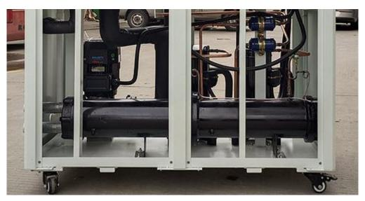
Shell and tube Condenser for water-cooled laser chiller
