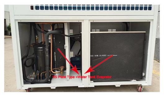
SS Plate Type+ Water Tank Evaporator
