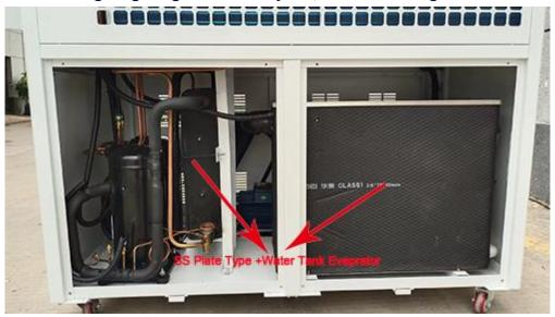
SS Plate Type+ Water Tank Evaporator
