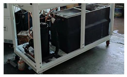
Coil in SS Water Tank Evaporator
