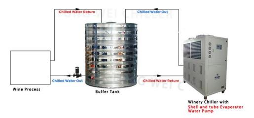
Air-cooled wienry Chiller Installation Drawing
