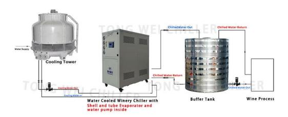
Water-cooled Wienry Chiller Installation Drawing
