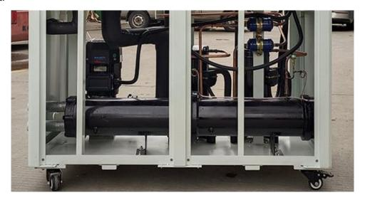
Shell and tube Condenser for water-cooled winery chiller
