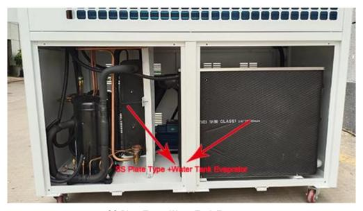
SS Plate Type+ Water Tank Evaporator
