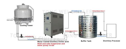
Water-cooled Distillery Chiller Installation Drawing
