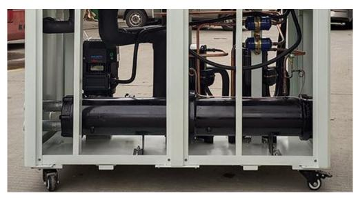
Shell and tube Condenser for water-cooled distillery chiller
