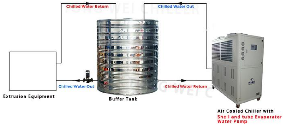
Air-Cooled Extrusion Chiller installation
