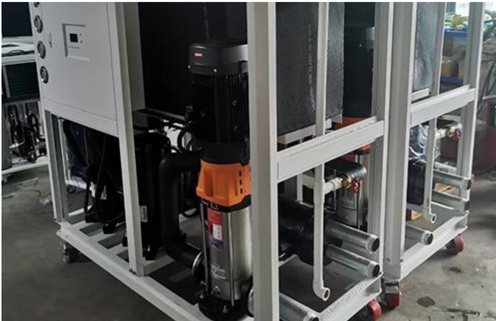
High Pressure Water Pump
