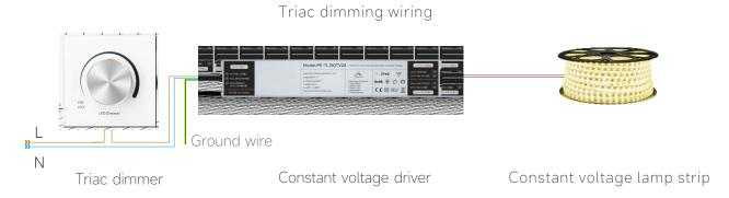
Note: 0-10V signal wire shall not be short circuited or grounded when using silicon controlled rectifier for dimming, otherwise dimming will be affected
