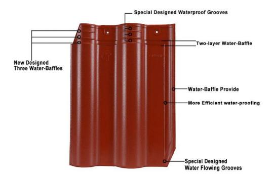
The flashing ceramic roof tile uses the unique waterproof structure. Its bottom structure of the roof tile allows rainwater to flow more smoothly and quickly, as the ceramic roof tile have a raised head that acts as a water barrier, preventing rainwater from flowing backward even on a horizontal roof. The unique dual waterproof structure makes the flashing ceramic roof tile have no worries whether they are used in strong wind and rainstorm areas or on slopes below 10  $^{\circ}$ C.
