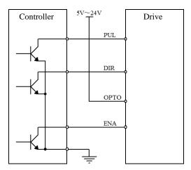
Note: OPTO is the common anode end of PUL/DIR/ENA. This drive only supports NPN controllers.
