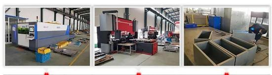
1.Laser cutting 2.Bending 3.Welding
