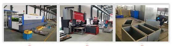
1.Laser cutting 2.Bending 3.Welding
