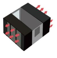
Cold aisle closure: The cold aisle is closed, and the inter-row precision air conditioners are arranged in the staggered positions of double-row micro modules or cabinets.
