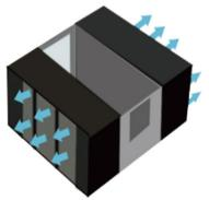
Hot aisle sealing: The hot aisle is sealed, and the precision air conditioners between columns are arranged in the staggered positions of double-row micro modules or cabinets. The temperature of the hot air flow in the sealed aisle is controlled (that is, the return air temperature control), and the cold air flow in the computer room is discharged into the closed aisle after passing through the server in the cabinet to cool the server.
