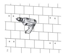
**Step2.** Fix the wall mount bracket to the wall with screws.
