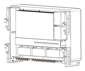
3. Pull the fan tray out slightly until the fan power connector is exposed, press down on the protrusion of the fan power connector and pull it out.
