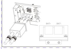
6. Tighten the sealing nut of the waterproof head
