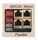
Rj45 Terminal Configuration of Meter/CT Communication
