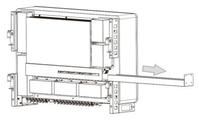
5. In the reverse order as above, reinstall the maintained fan back to the converter and restart the system
