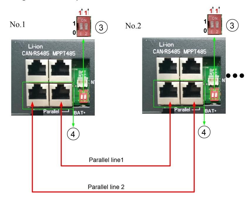
■ If there are more than two inverters parallel in your system, only two of longest distance of need to be dialed toward "on "position: ¹¹¹¹, and others keep off: ¹¹¹
