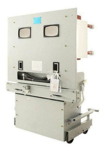
ZN85-40.5/31.5-300 is a HV indoor vacuum circuit breaker working as a protection and control unit of power grid equipment and industrial electric equipment in power system of rated voltage from 40.5KV. It meets the requirements of GB/T1984-2014 (AC HV circuit breaker) and JB355-1996 (3.6KV-40.5KV indoor AC HV vacuum circuit breaker). It can be used in switchgears of KYN61.
