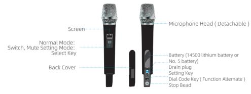
The product adopts hybrid circuit technology, can use two 1.5V ordinary batteries or two 3.7V, 14500 rechargeable lithium batteries, can continue to speak for 10 hours or continuous 24 hours of standby work, and the use of unique encryption technology to ensure that the meeting information security; equipped with LCD display, can real-time display call volume, call status, with independent gain adjustment, speech timing function, support two Role definition: VIP \ listed.
