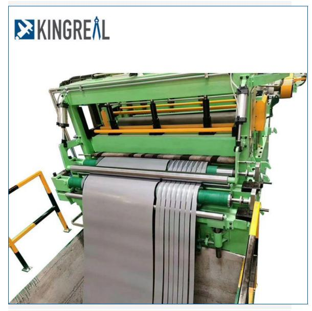
A silicon steel coil slitting machine is a production and processing machine that cuts rolls of silicon steel coil to a certain width and then rolls them into coils under a certain coiling tension.
