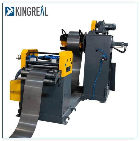
The KINGREAL combine decoiler and straightener machine integrates uncoiling and leveling functions, which can reduces the material loop between the uncoiling and leveling process. The uncoiling speed is controlled by a photoelectric switch, and there is no damage to the surface of the material during operation.
