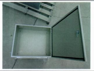
After IPX5 test picture of EUT
