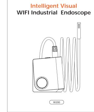
W200 is an wifi industrial endoscope camera with HD camera. The product transmits WiFi signal, the mobile phone connects to the product WiFi, and the picture is displayed on the APP. This product is equipped with a small diameter HD camera with LED auxiliary lighting. The camera adopts a high-sensitivity chip, which can beused normally even in a dark working environment.
