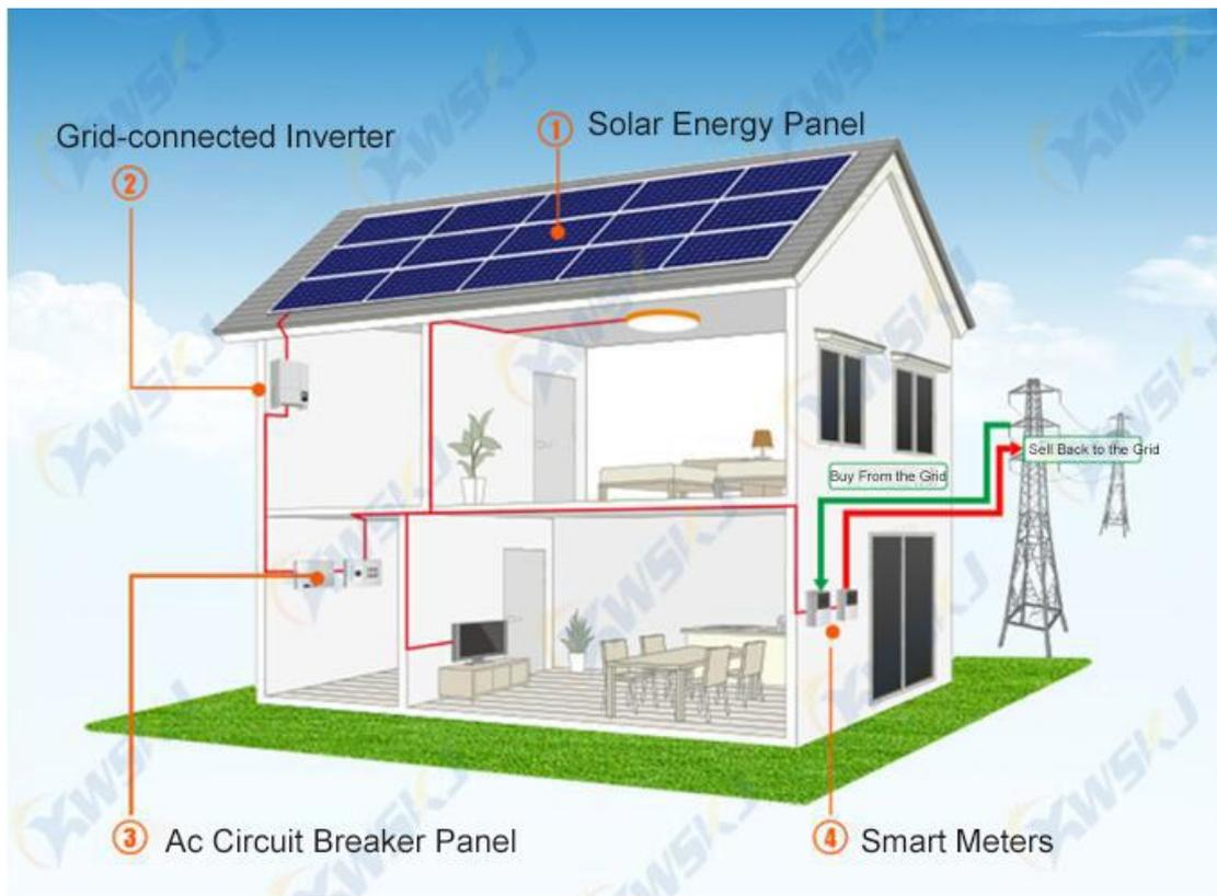
The PV on-grid power generation system consists of PV modules, PV combiner boxes, PV on-grid inverters, metering device and power distribution system. The energy of solar energy is converted into DC power through PV modules, and then the DC power is converted into sine wave AC power with the same frequency and phase of the grid through the on-grid inverter power supply and input to the grid.
