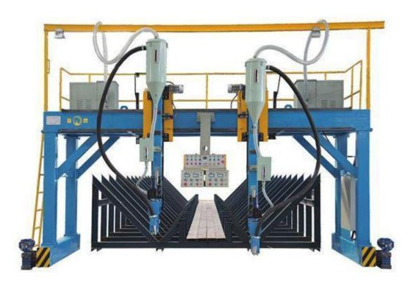
H beam welding machines in Gantry type MZG
