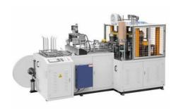
**Big Size Paper Bowl Making Machine** This Big Size Paper Bowl Making Machine is a multi-station automatic machine that produces paper soup bowls, instant noodle bowls, etc. Ideal equipment for large-capacity caliber or other food containers. Power supply: 220V-380V free choice. Automatic control adopts light-controlled non-contact switch. Model:YB-W35
