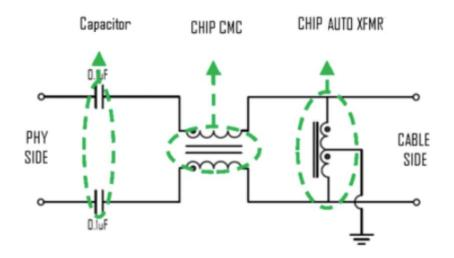
Capacitor+Chip Common Mode Choke+Chip Auto Transformer Solutions (Shortly named Cap+CMC Solution)
