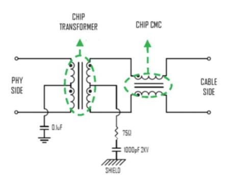
Chip Transformer+Chip Common Mode Choke Solutions (Shortly named X'fmr+CMC Solution)
