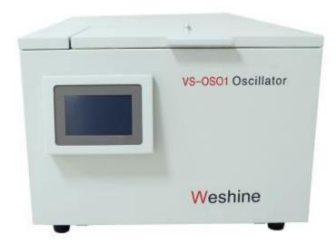
The Oscillator heats and shocks the transformer oil to extract the gases from the transformer insulating oils automatically. The temperature and times can be set. Put the 40ml oils into the 100ml-injector, and then put 8 injectors at max into the oscillator to start the extraction works.
