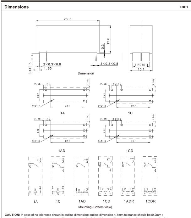
**CAUTION:** In case of no tolerance shown in outline dimension: outline dimension ≤1mm,tolerance should be±0.2mm; outline dimension >1mm and ≤5mm, tolerance should be±0.3mm; outline dimension >5mm, tolerance should be±0.4mm.
