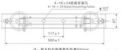
注: 瓷支柱外绝缘爬电距离600mm。 Note: The creepage distance of the outer insulation of the porcelain pillar is 600mm.
