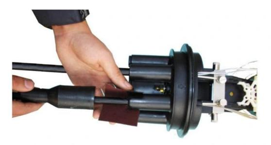
(9) Bound and even the heat-shrink part with aluminum paper to avoid burn caused by high temperature of blast burner.
