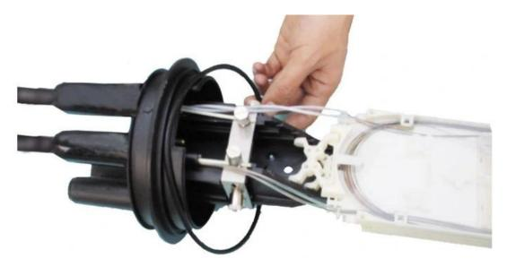
(13) Put the barrel on the base.
