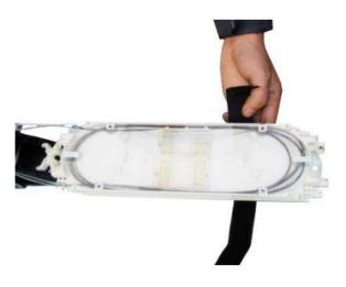
(7) Sealing of the cable and the base: clean the entry ports and cable with 10cm long by scrubber.
