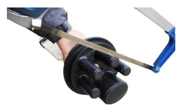
(2) Strip the cable as the requirement of installation, and put the heat-shrinkable tube on.
