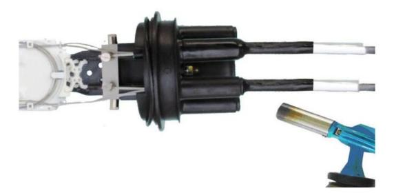
(11) Usage of branch folk: when heating the oval entry port, folking the heat-shrinkable tube to separate the two cables and heating it follow the steps above.
