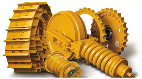
Heavy duty track roller is made of shell, bronze bushing, collar, seal, lock pin, plug, shaft. It is made by forging, machining, heat treatment, assembly, painting etc. The quality and working life for heavy duty track roller is depends on the quality of raw steels, the hardness of rail surface, the depth of hardness layer, the quality of seal group etc.
